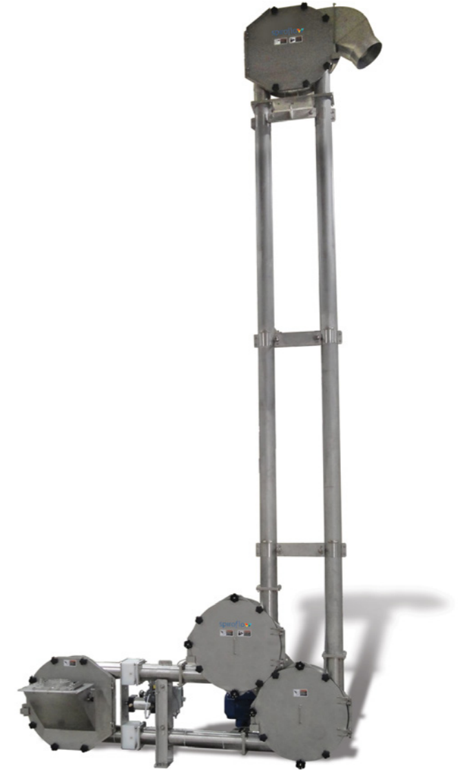
This aero-mechanical conveyor is a balanced venting system operates below 85dBA and conveys at a rate from 400 to 1,840 cubic ft/hr.
