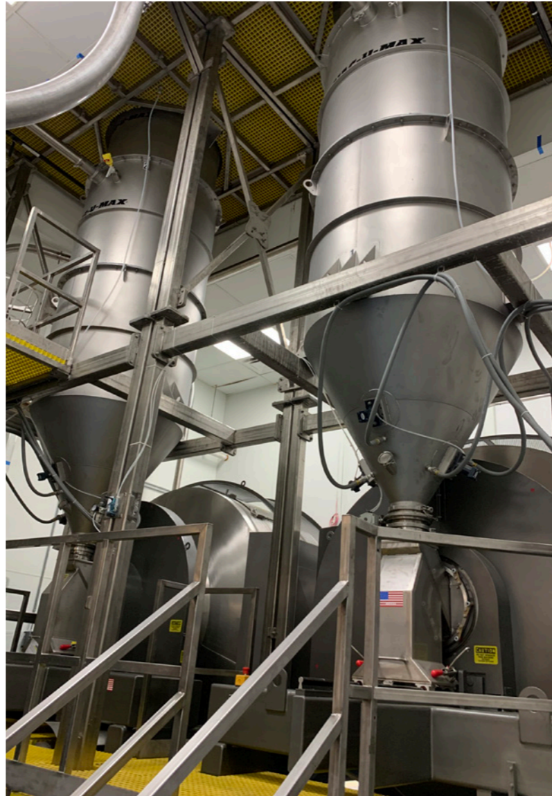
Vac-U-Max 160-cu-ft CIP filter receiver conveys product to CIP rotary batch mixer, increasing productivity while reducing sanitizing downtime from by over 75% (photo courtesy of Vision Conveyor)
