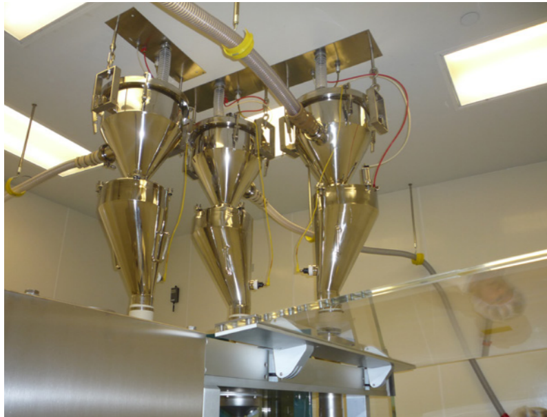
Sanitary vacuum conveyor keeps tablet press filled in pharmaceutical environment.
