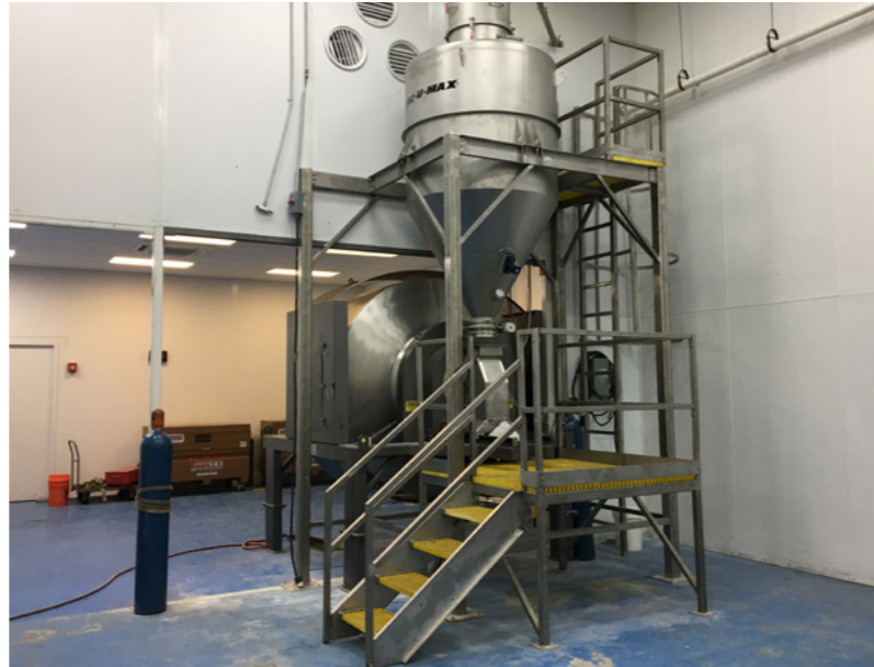
Vac-U-Max 80-cu-ft vacuum receiver system holds a full batch of ingredients ready for the rotary batch mixer at a leading beverage producer (photo courtesy of Vision Conveyor)
