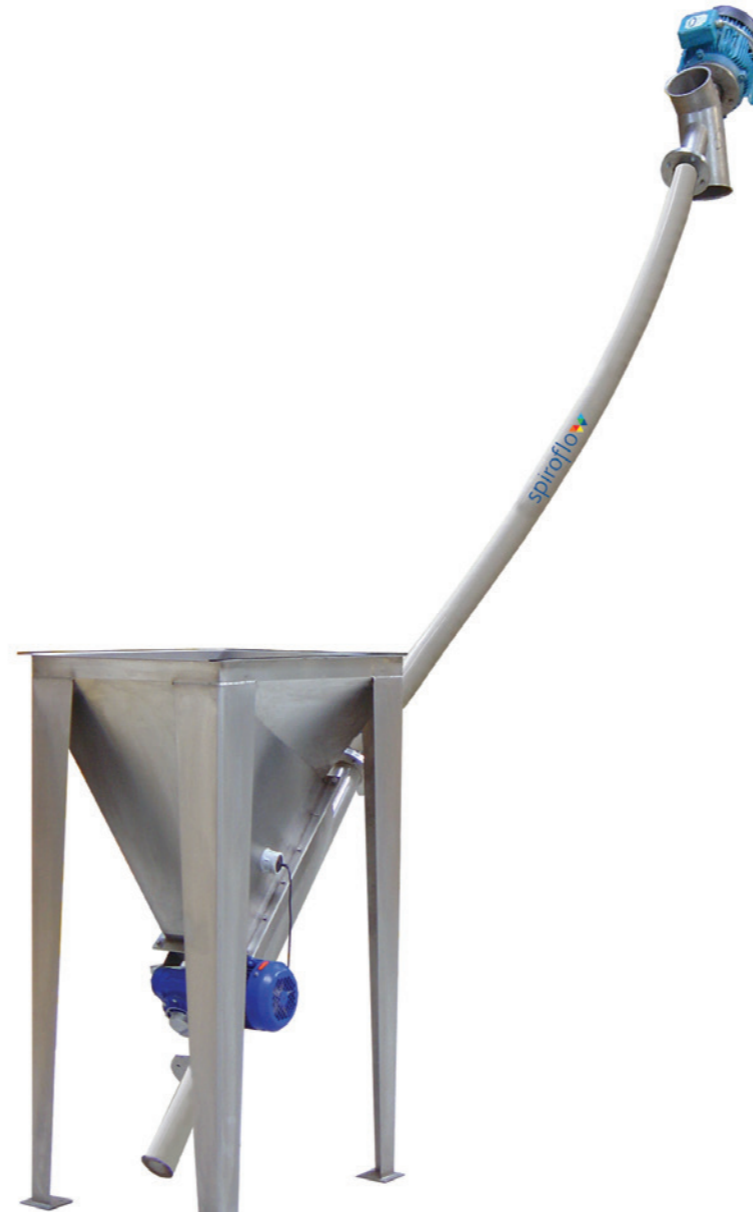
This flexible screw conveyor is a simple, low-cost solution comprised of a stainless steel spiral rotating within an UHMWPE food-grade tube.
