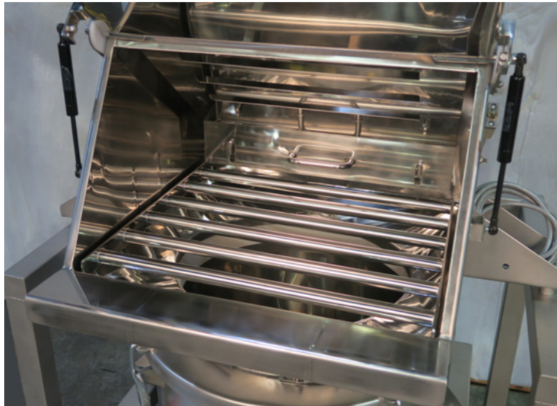
Sanitary stainless-steel bag dump station for nutraceutical manufacturer with grate magnet and highly polished interior is ideal for food processing applications.
