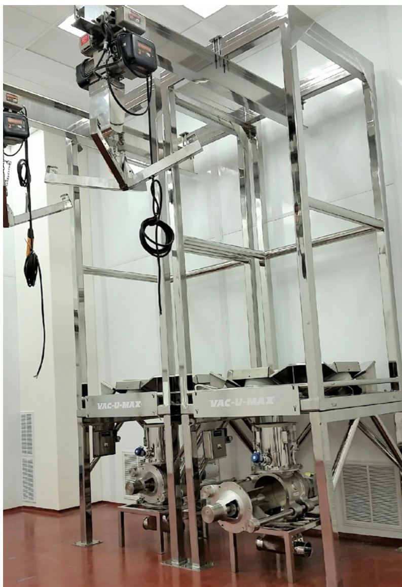
Highly-polished bulk bag unloader with food-grade hoist and sanitary rotary valve for baby formula producer
